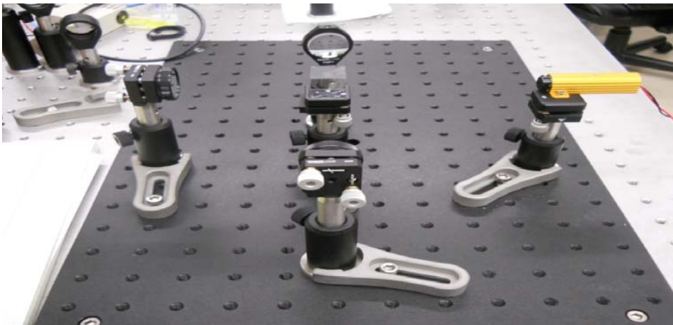
Figure 2: Sample Michelson Interferometer Using Permanent Materials that I have assembled
