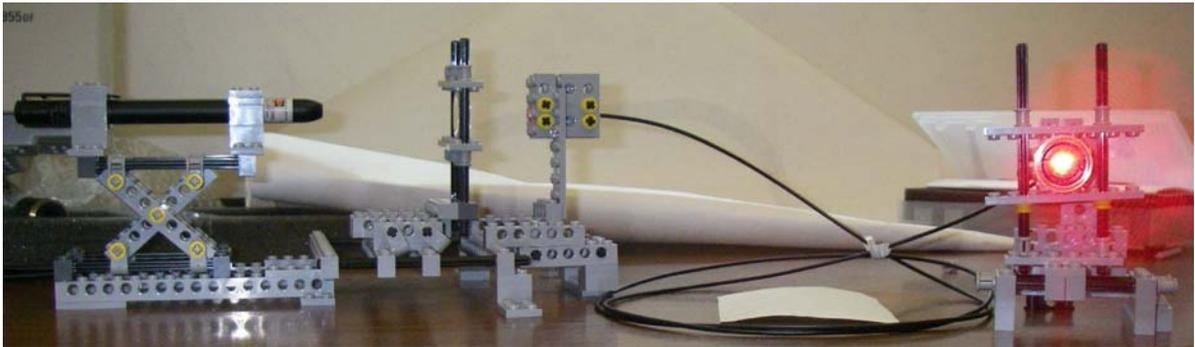
**ADA Description:** A laser being guided into and out of a fiber using LEGO optical mounts
