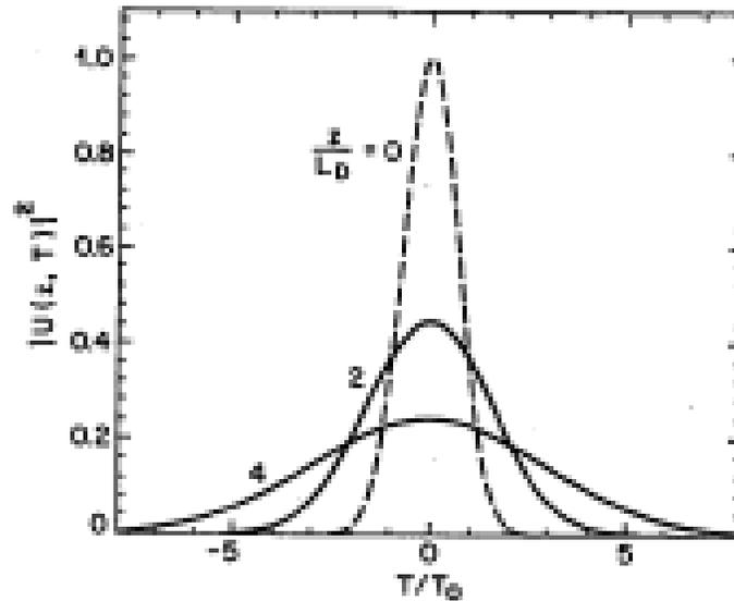
**Figure. 2.7** This Figure shows dispersion-induced broadening of an input Gaussian pulse for propagation distances  $z = 0, 2L_D, 4L_D$ .
