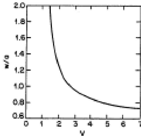
**Figure. 2.2** Normalized best-fit Gaussian spot size ( $w/a$ ) as a function of the V-parameter.
