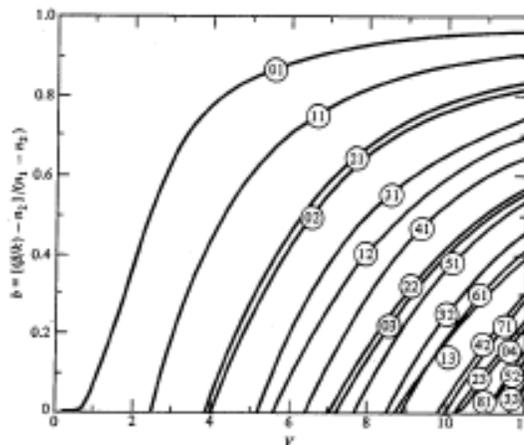
**Figure. 2.3** Normalized propagation parameter  $b$  versus V-parameter for various LP<sub>*jm*</sub> modes with the *jm* values shown in the circles. The fundamental mode corresponds to the LP<sub>01</sub> mode.
