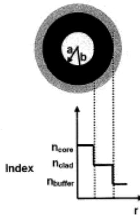
**Figure. 2.1** Step-index fiber geometry.
