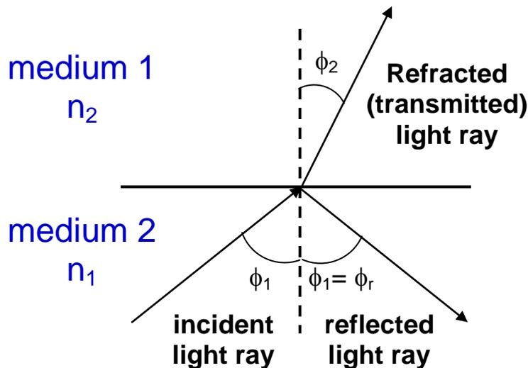
**Figure 2.8:** *Reflection and refraction at an interface between two media. The refracted angle is given by Snell's law.*
