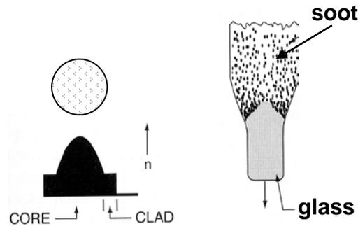
Figure 2.15: VAD preform index profile (left) and sintered preform rod (right).
