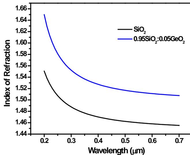
**Figure 2.4:** *Refractive index dispersion for silica glass and for germanosilicate glass over the visible portion of the optical spectrum.*
