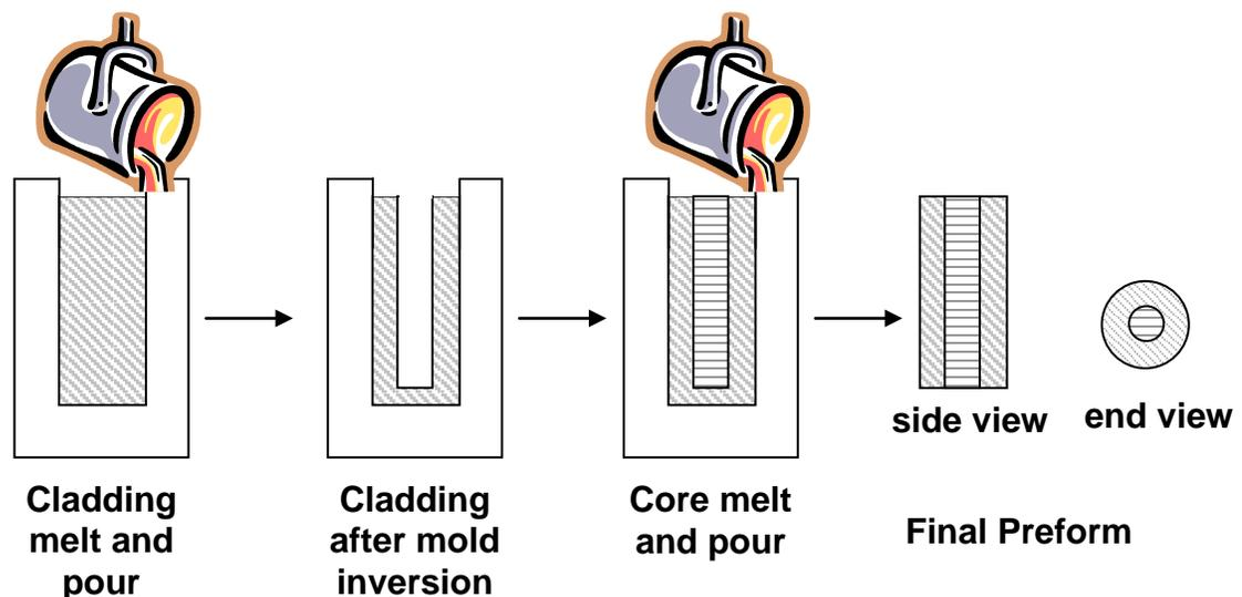
*Figure 2.18: Schematic of the build-in casting technique*
