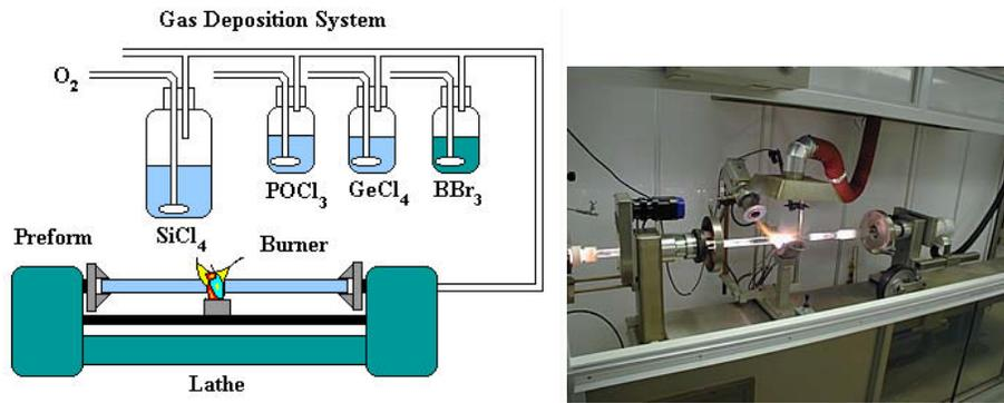
**Figure 2.16:** MCVD deposition apparatus.
