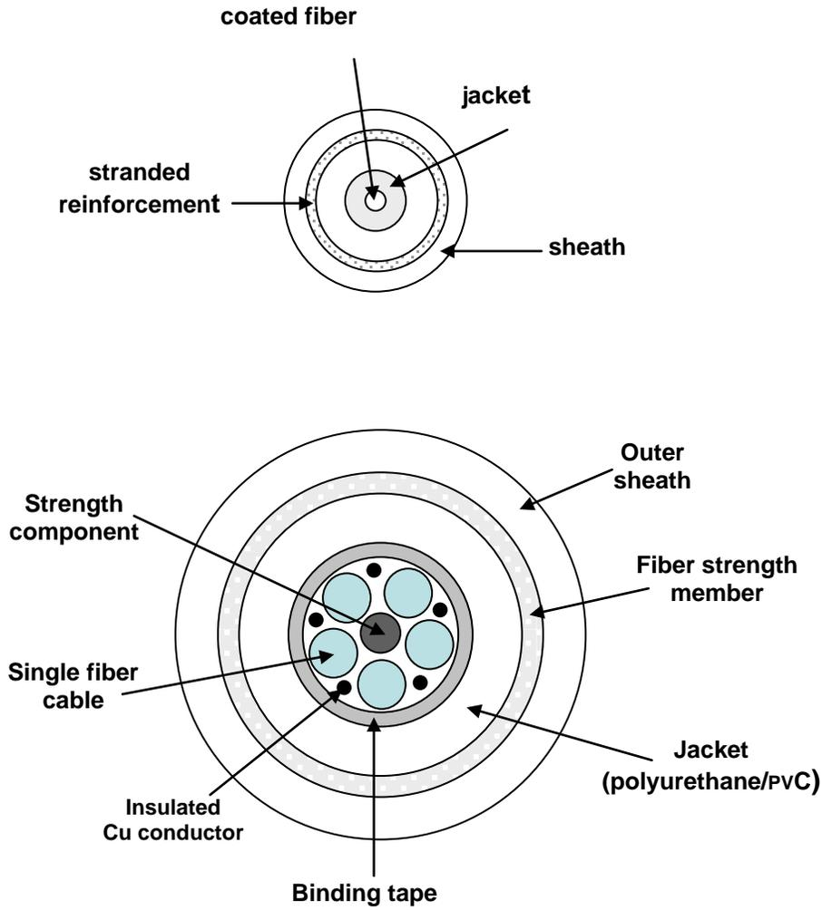
*Figure 2.21: A single-fiber cable design (top) and a multi-fiber cable design (bottom).*
