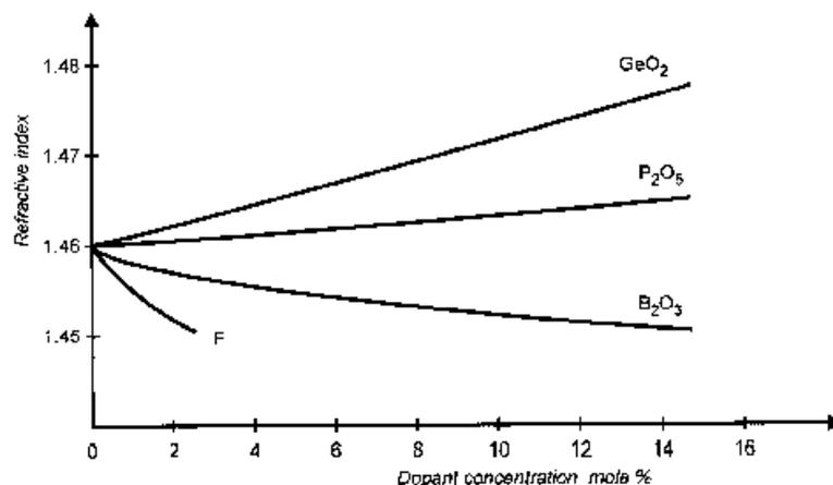
**Figure 2.7:** *Dependence of the visible refractive index of doped silicate glasses on composition.*
