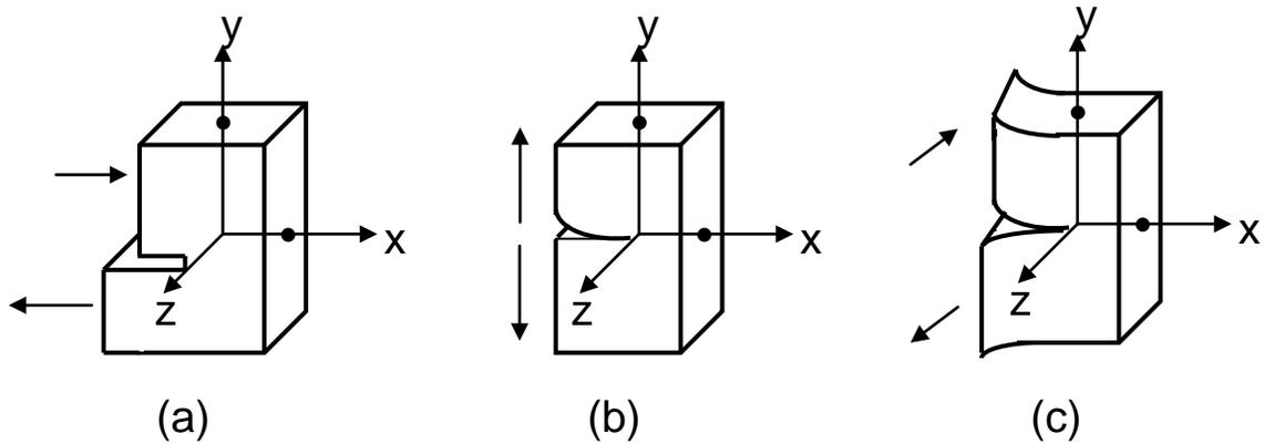
**Figure 2.6:** Different modes of crack propagation (a) sliding, (b) opening, and (c) tearing.
