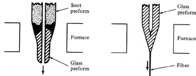
**Figure 2.13:** Preform rod heating and collapse followed by final fiber draw to produce optical fiber.
