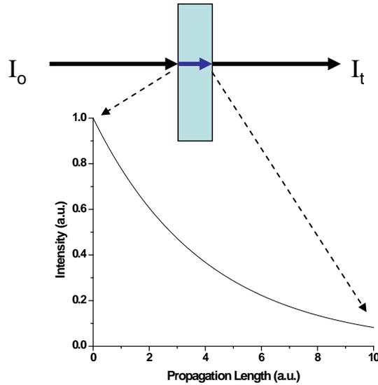
**Figure 2.3:** Exponential decay of transmitted intensity in an absorbing material.
