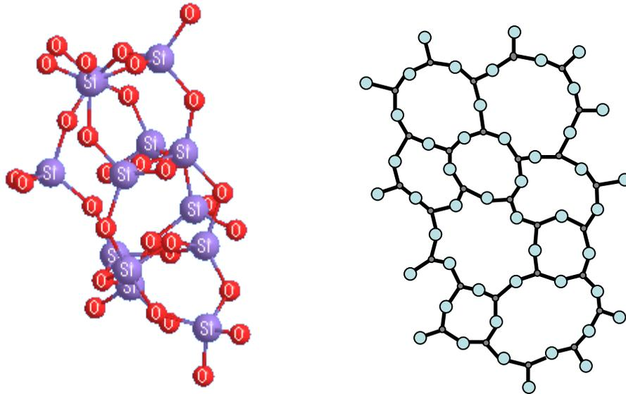
**Figure 2.1:** *Three and Two-dimensional illustration of silica tetrahedral network in a glassy structure. Note that the fourth oxygen atom in each tetrahedron will be connected to each silicon atom out of the plane of the drawing, thus forming the full three-dimensional network.*
