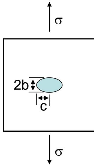
**Figure 2.5:** Elliptical flaw in a glass plate that is placed under tension.
