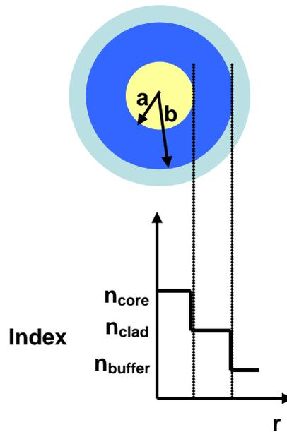
*Figure 2.9: Step-index fiber geometry.*
