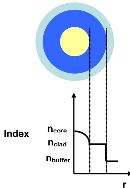
**Figure 2.10:** Gradient-index fiber geometry.
