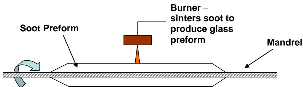
**Figure 2.12:** *Outside Vapor Deposition technique.*
