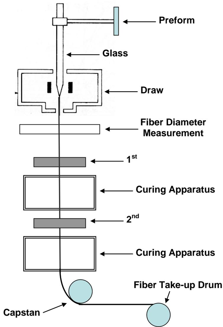
*Figure 2.20: Schematic of fiber draw tower.*
