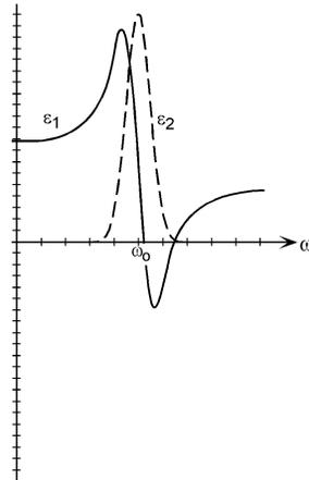
**Figure 2.2:** *The real and imaginary parts of the complex dielectric function with frequency.*
