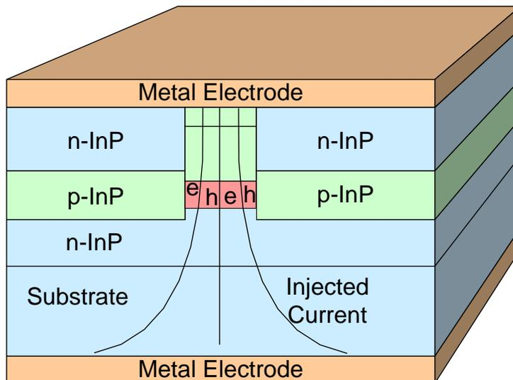
Figure 6.27: Current flow in a buried heterostructure semiconductor laser.
