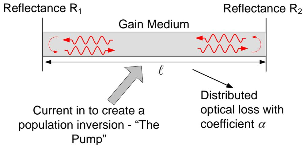
**Figure 6.20:** Electrical current is the pump source for most semiconductor lasers. Optical loss is distributed throughout the gain medium.
