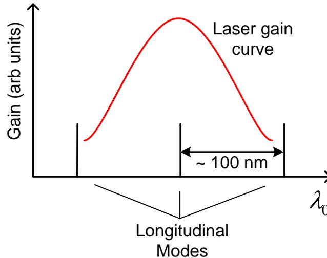
**Figure 6.35:** Only one longitudinal mode falls under a VCSEL gain curve.
