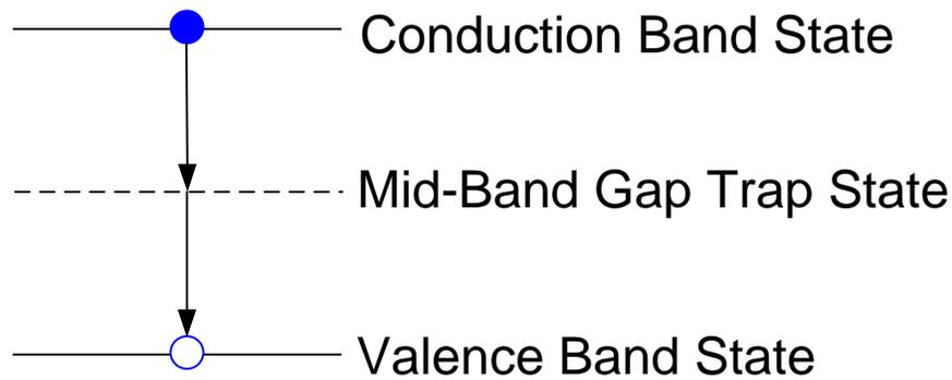
**Figure 6.15:** Shockley-Read-Hall type recombination of an electron with a hole.
