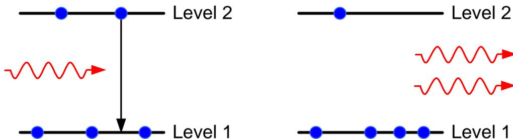
**Figure 6.5:** A Photon stimulates a particle to a lower energy level, creating a second photon.
