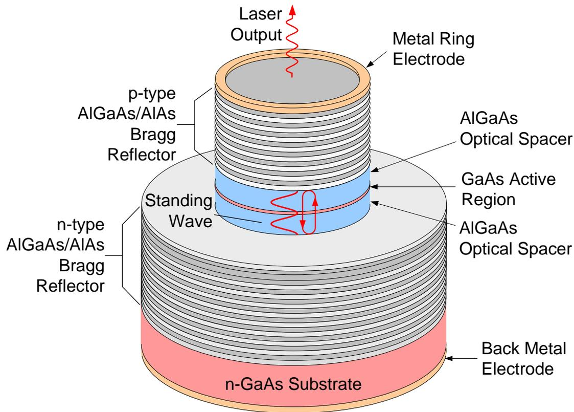
**Figure 6.34:** A GaAs surface emitting laser.
