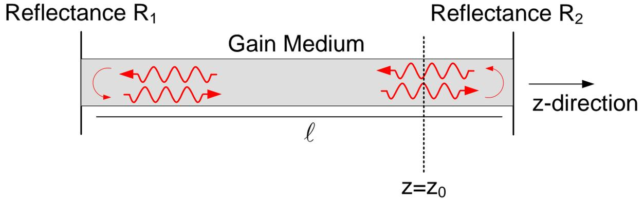
**Figure 6.24:** To establish a phase condition for lasing we examine the phase of the circulating light at the plane  $z = z_0$ .
