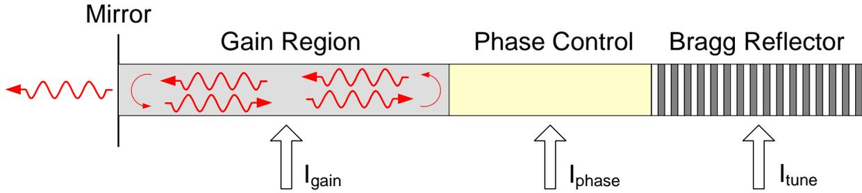
Figure 6.32: A tunable distributed Bragg reflector laser.
