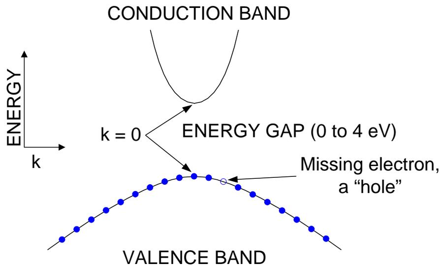
**Figure 6.9:** Valence and conduction bands in the energy versus momentum picture.
