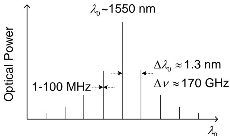
**Figure 6.25:** A semiconductor laser can operate in several longitudinal modes.
