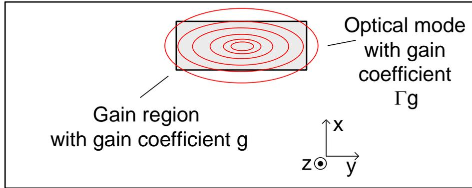
**Figure 6.22:** The overlap of an optical beam with the gain region defines the confinement factor.
