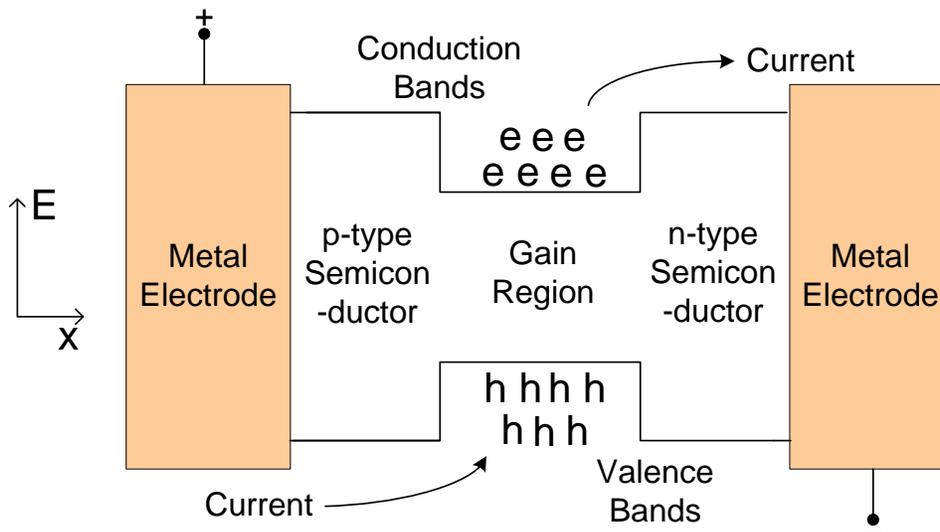
**Figure 6.14:** A double heterostructure, p-n junction for creating a population inversion in a semiconductor.
