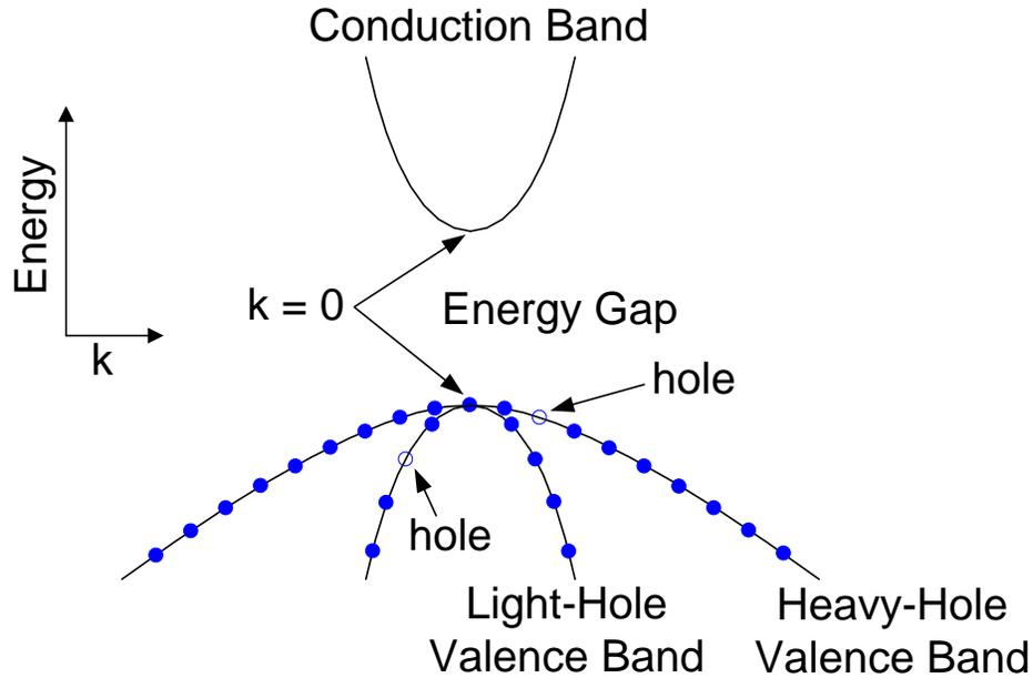
**Figure 6.10:** Energy versus momentum picture with two valence bands.
