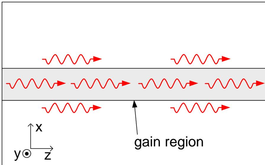
**Figure 6.21:** Semiconductor lasers contain light outside of the gain region.
