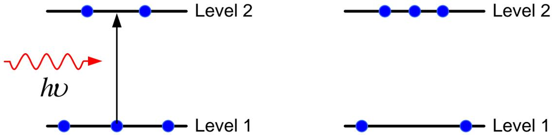
**Figure 6.4:** A photon is absorbed as a particle is excited from energy level 1 to energy level 2.
