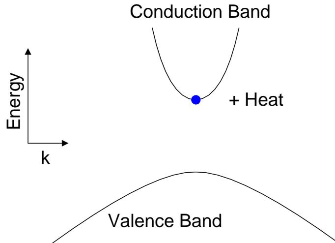
*Figure 6.17: A CCCH Auger process removes an electron-hole pair from the semiconductor and converts the energy of the pair into heat.*
