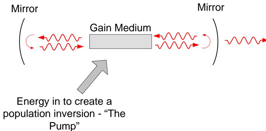
**Figure 6.18:** Lasers have a gain medium, a pump, and mirrors.
