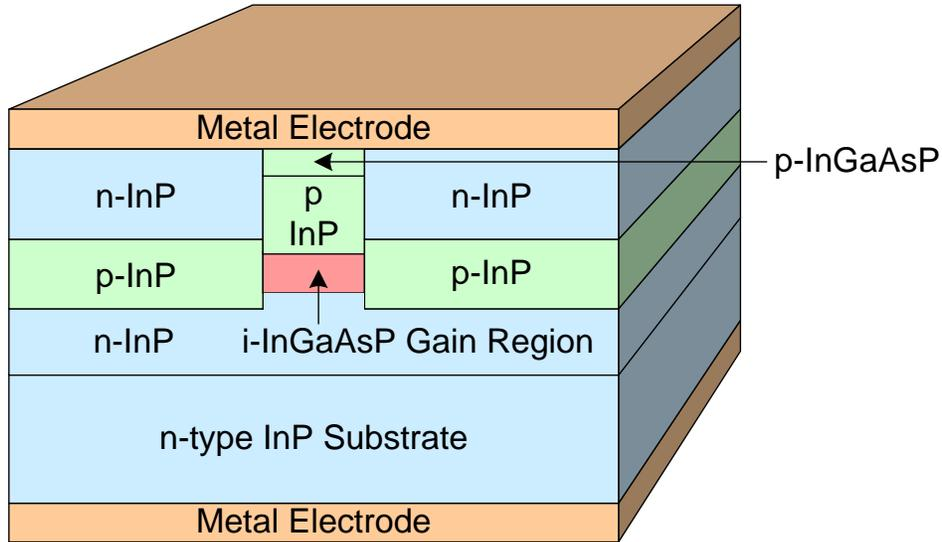
Figure 6.26: A buried heterostructure semiconductor laser.
