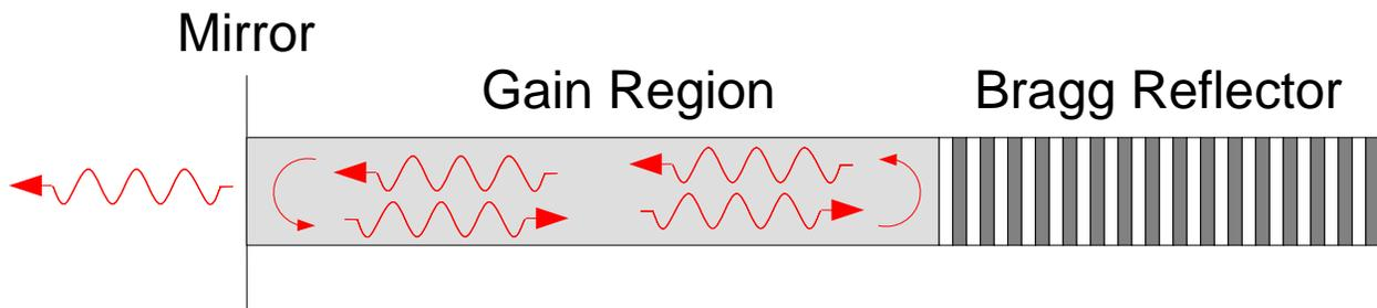
**Figure 6.31:** A single mode distributed Bragg reflector laser.
