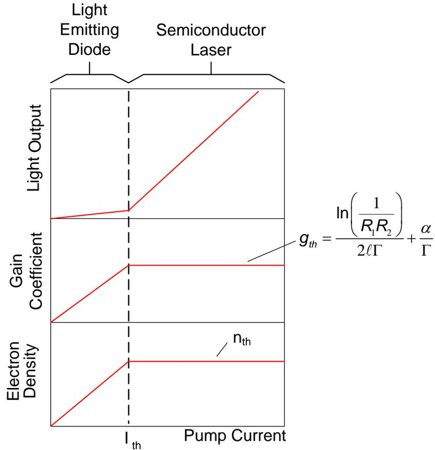
**Figure 6.23** Above threshold the electron density,  $n$ , and gain coefficient,  $g$ , are clamped at values determined by the gain-loss balance equation while light output increases linearly.
