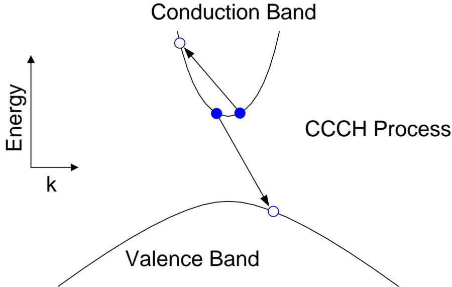
*Figure 6.16: A CCCH Auger recombination process.*
