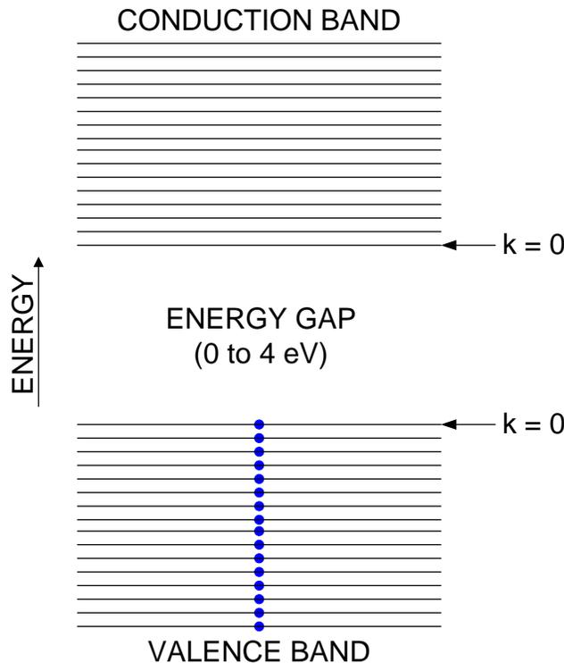
Figure 6.8: Energy bands in a semiconductor
