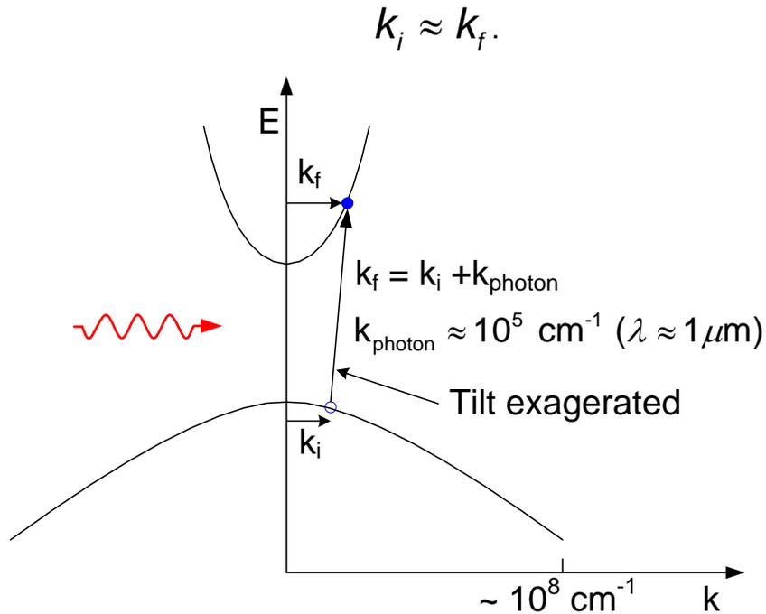
Figure 6.11: Optical transitions in semiconductors are “vertical”.
