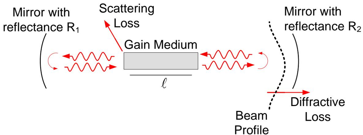
**Figure 6.19:** Gain and loss mechanisms for a laser.
