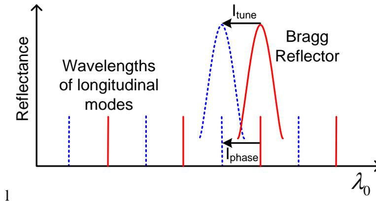
Figure 6.33: The phase current positions a longitudinal mode in the high reflectance band of the Bragg reflector.
