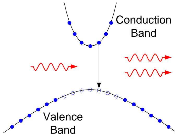
Figure 6.12: A simple picture of population inversion in a semiconductor.
