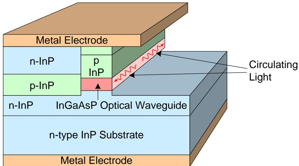
**Figure 6.28:** The InGaAsP gain region has a high refractive index than the surrounding material and forms the core of an optical waveguide that confines light that circulates from end to end.
