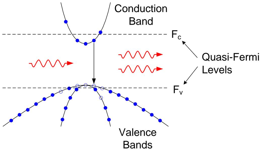
**Figure 6.13:** A more precise picture of population inversion in semiconductors includes quasi-Fermi levels.
