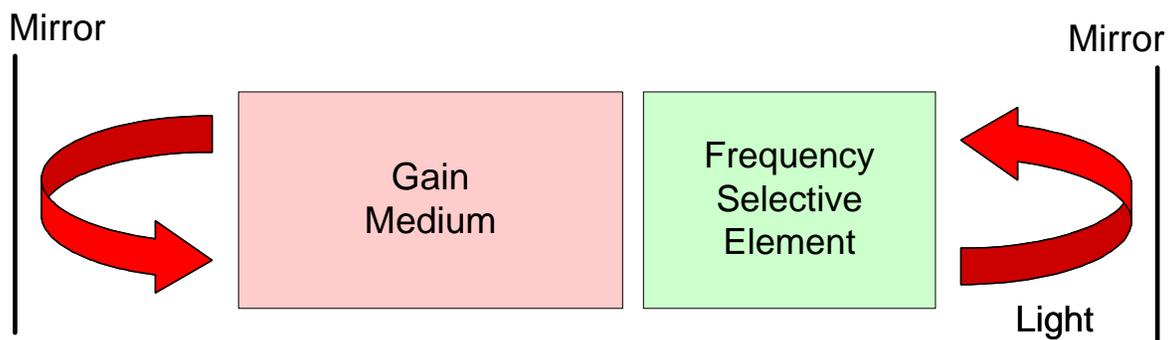
**Figure 6.29:** A frequency selective element is introduced into a semiconductor laser to narrow the output spectrum.
