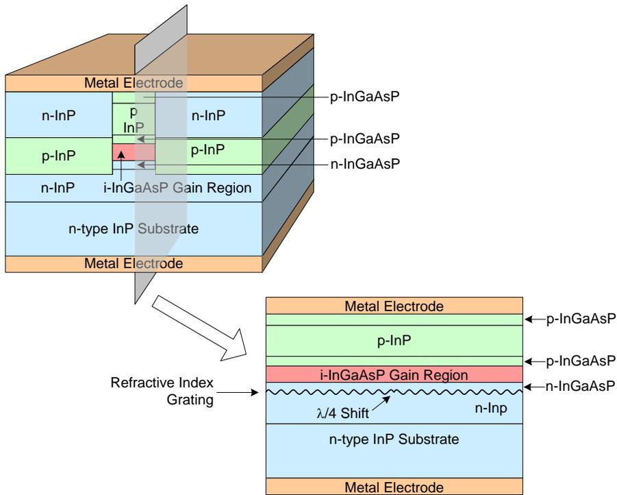
**Figure 6.30** A cross section of a distributed feedback (DFB) semiconductor laser.
