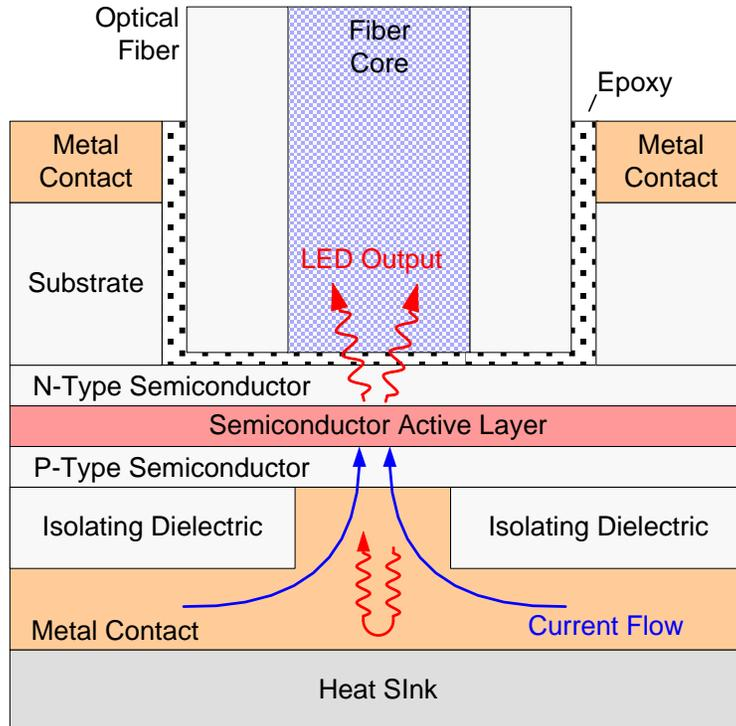
**Figure 6.36:** A light emitting diode (LED).
